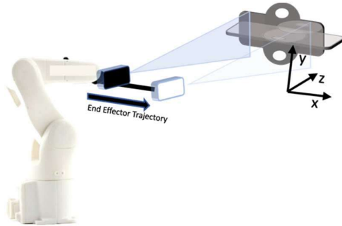
Fig. 3 Laser triangulation system on the robot end effector for 3D measurements
