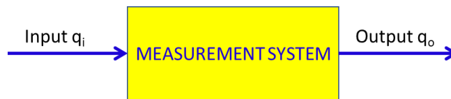
Figure 1: Block representation of a measurement system
