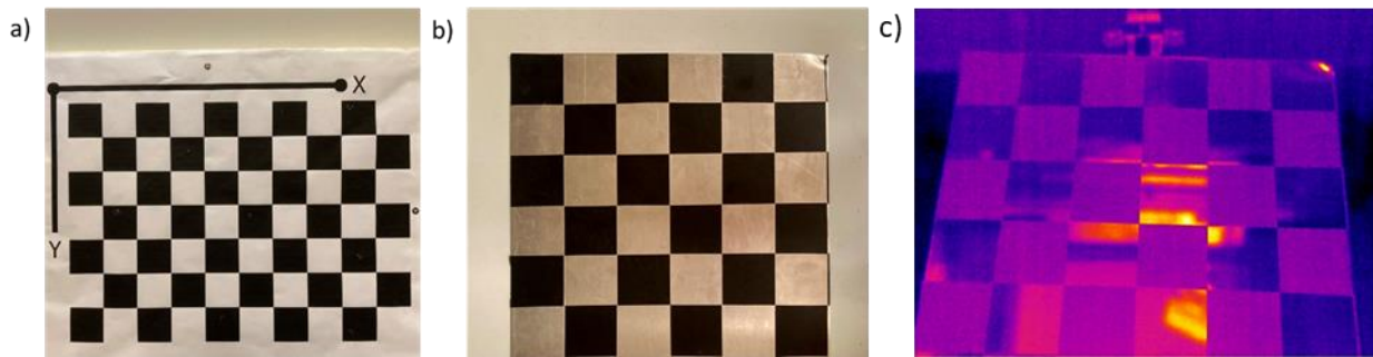
Figure 27: a) Checkerboard for visible systems, b) checkerboard for infrared systems, c) infrared image of the checkerboard for infrared systems
