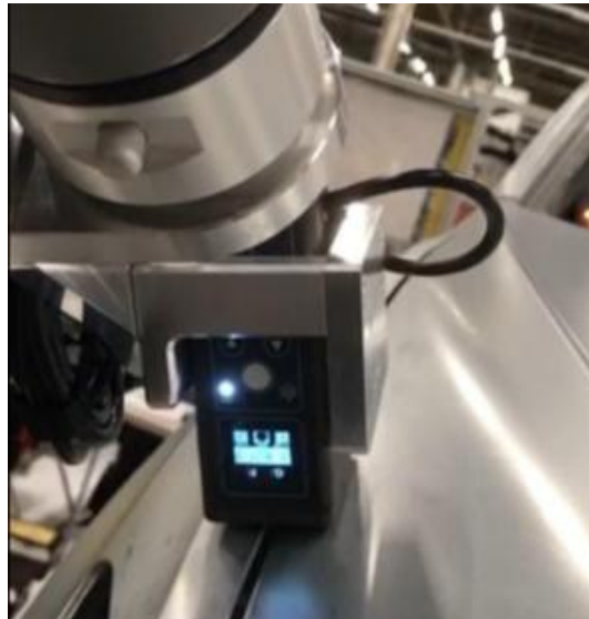
Figure 5: NDI#8 integrated in the collaborative robotic arm
